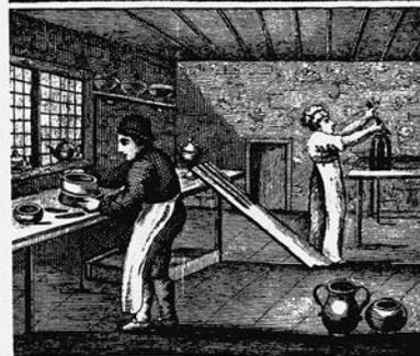
*"Pressing" or "Squeezing", which is making jugs, tureens &c. of the clay, ready for being fired.*
